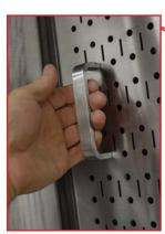
Using handles (2) located on right & left, lift & pull to remove backsplash
