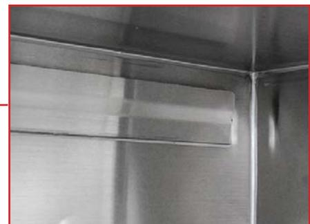
Mounting bracket located behind backslash secures pegboard to station
