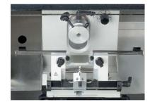
the CE knife holder. The edges of the glass insert are manufactured using a special procedure to make them more durable and fracture-resistant. All four edges of the insert can be used.
