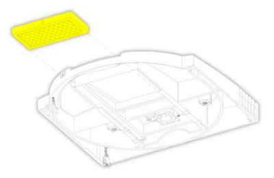
Fitting the filter into the instrument
