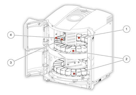
Gemini AS (inside view) 1 Heater/Holding stations, 2 Reagent pots, 3 Pick-up arm, 4 Water wash stations.
