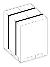
Remove the packing bands from around the outside of the packaging.
