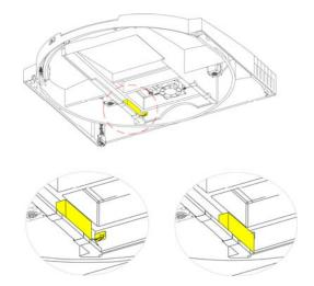
Step 3: Use the rectangular block (provided in the kit) provided to activate the filter sensor by fitting the block as shown. Ensure that the rectangular block is securely located at the back of the filter channel otherwise it will not activate the filter sensor.
