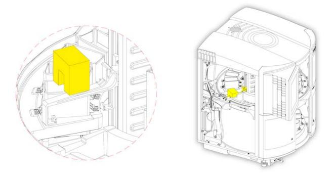
Remove the small foam block securing the pick up arm. Remove the baskets from the front pots and keep them for later use.
