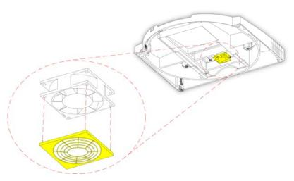
Step 2: Remove the filter (if fitted) from inside the Gemini AS top cover. Attach the fan guard to inlet side of the extractor fan by firmly inserting the plastic lugs into the holes at the corners of the fan.
