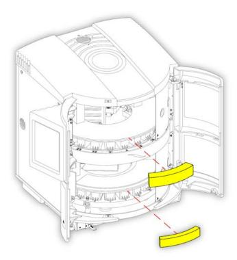
Open the instrument's main doors and remove the inner foam pieces from behind the sliding doors.
