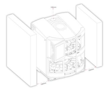
Ensure adequate clearance of at least 100 mm (4 in) for fan inlets
