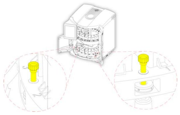
Releasing the locking knobs to rotate the lower turntable
