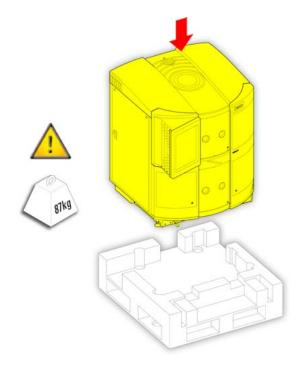
Placing the instrument on its base
