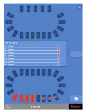
The Load Set screen, pots 18, 19 and 20 are still to be loaded with xylene
