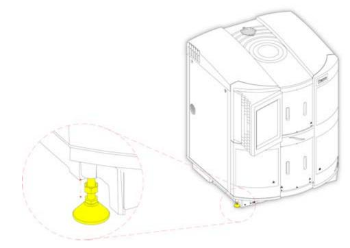
Levelling the instrument
