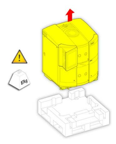
Lift the Gemini AS off the wooden packaging base and place the instrument onto a bench.
