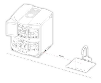
Position the instrument no more than 1.8 m (6 ft) from a drain and water supply
