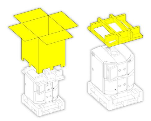
Remove the outer packaging and then remove the foam inner packaging.
