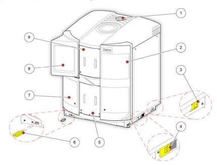
Gemini AS (outside view) 1 Air extraction outlet, 2 Main access door, 3 Battery isolation switch, 4 Mains power connector and switch, 5 Unload door, 6 USB port, 7 Main access door, 8 Touchscreen, 9 Load door.
