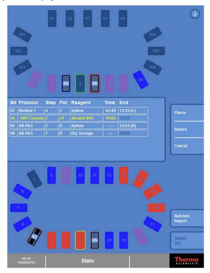
The Batch Monitoring window shows the progress of each batch
