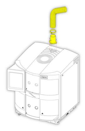
Step 1: Fit the flexible ducting over the mounting bracket and secure using the clip provided. Fix the mounting bracket to the Gemini AS top cover over the fan outlet grille using the four screws and gasket provided.
