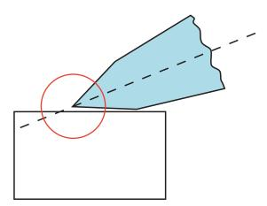
An angle, which is too steep, is also unfavorable as the knife/blade might vibrate too much while sectioning. The so-called "chatters" appear on the block surface as well as on the sections as parallel stripes having negative effects on the microscopical evaluation.
