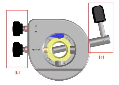
To bring the specimen into the desired position, move the clamping lever [a] towards the front.
