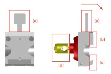
• To insert or remove the cassette from between the fixed [b] and movable [c] jaws, pull the lever [a] to the front (in the direction of the arrow).
