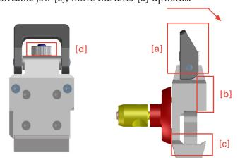
• To adjust the size of a cassette size which is not to the norm, use the adjustment nut [d].
