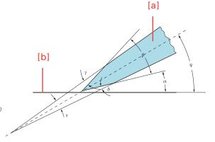
The knife/blade must never be placed on an angle that is too flat since the knife/blade does not cut into the block at all this way. Only the rear side slides over the sectioning surface.
