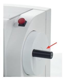
• To unlock the handle, turn off the motorized cutting drive and press the interior locking knob of the hand wheel handle.
