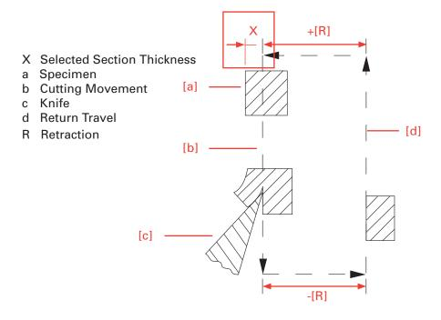
The yellow LED Retraction lights up. If desired, the function <retraction> can be turned off.
