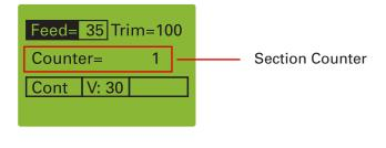
The section counter adds up the number of sections produced. After each downward movement of the specimen holder, the number on the section counter increases by 1.
