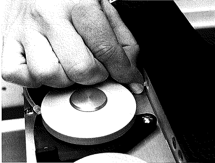
Figure 2-4 Attaching Pump Tubing to Nipple
