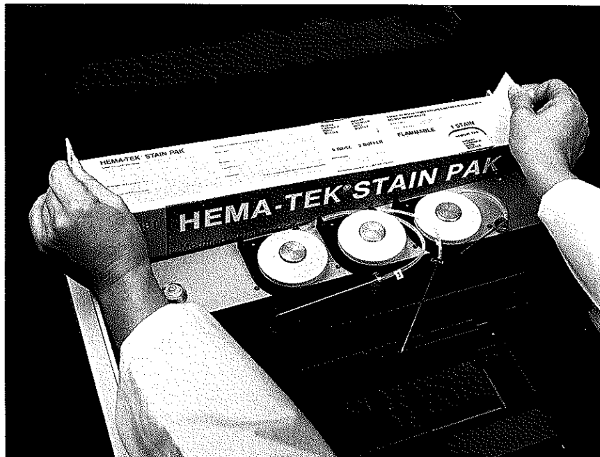
Figure 2-5 Installing the Stain Pak
