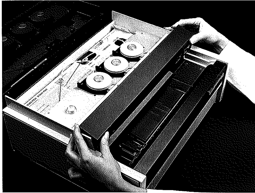
Figure 6-5 Raising the Circuit Board Cover
