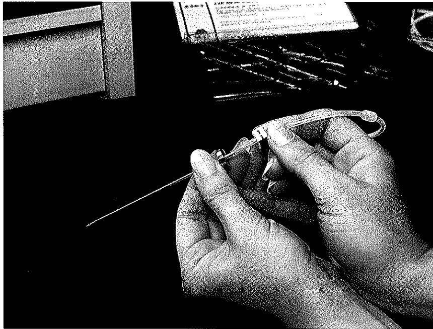
Figure 2-2 Attaching Pump Tubing To Cannula
