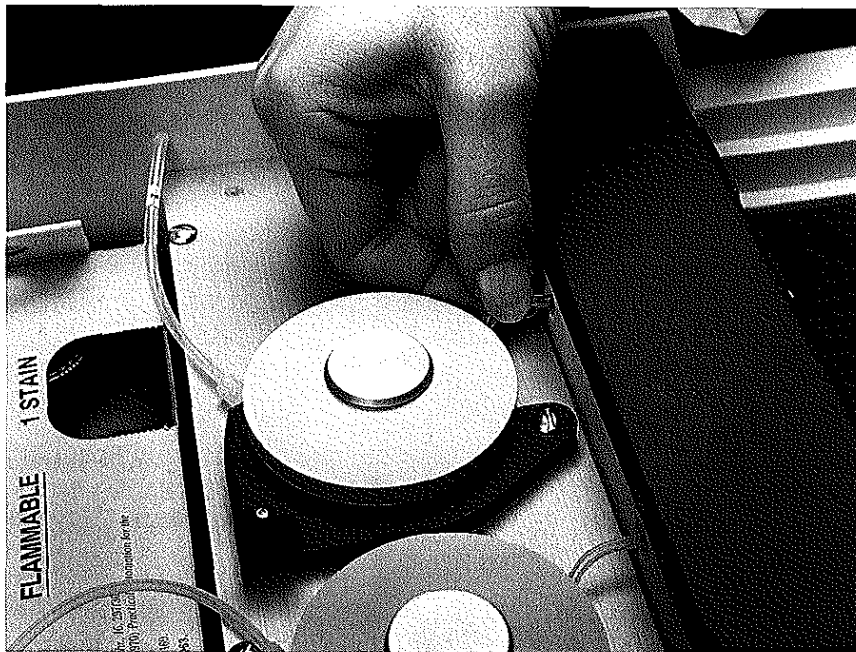
Figure 8-6 Removing Tubing from Nipple
