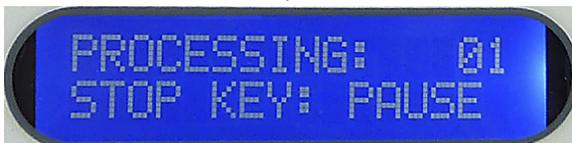
If a staining run is already underway and more slide carriers are to be inserted, press the PAUSE/STOP key **Only ONCE**.
