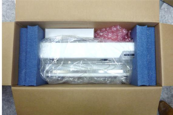
3. Use the molded foam pads to pull the Stainer out of the box and place it on a firm laboratory bench.
