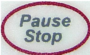
Pressing the PAUSE/STOP key allows the operator to exit the setup menu without changing the parameter currently being displayed.
