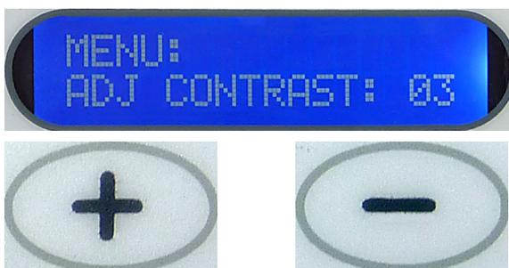
The contrast on the Liquid Crystal Display (LCD) may be adjusted to the preference of individual operators by pressing the INCREMENT (+) or DECREMENT (-) keys, followed by the ENTER key.
