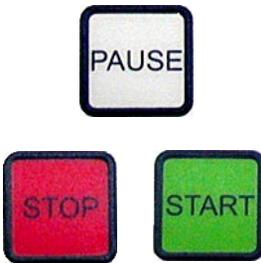
**PAUSE** has the same function as described in section 5.3 (as long as the bath guide is not pulled out, the slide rack is removed by the TS5025 if the coverslipping process is continued or concluded).
