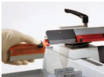
Safer insertion of disposable blade
