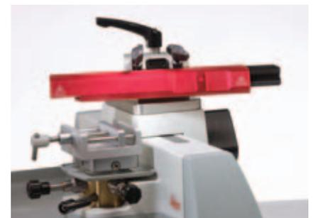
Knife holder SN for standard knives or disposable blade rails
