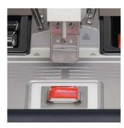
The large Peltier element cold spot is designed to assist tissue orientation even with large Super Mega Cassettes.
