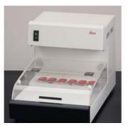
The Leica EG1150 C cold plate is held at a constant temperature of - 5 °C. The easy to load, large capacity plate can hold in excess of 70 standard cassette molds. An optional cover reduces frost build up in high humidity environments. Additionally, the cold plate can be used as a stand alone unit for pre- cooling blocks prior to sectioning.
