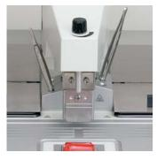
The heated, removable forceps holder is easily accessible from either side.
