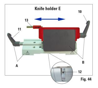
Lateral displacement (only for knife holder E) The lateral movement feature of the knife holder base enables the use of the entire length of the blade or knife, eliminating the need for readjusting the knife holder. The knife holder E consists of a segment arch A (with lever (11)) and the clamp mount B (with lever (10) and ejector (13)). The extreme left and right positions as well as the middle position are each marked with a notch point.
