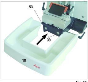
Push the section waste tray (18) from the front to the microtome base plate (53) until it is held in place by the two magnets (39) (on the front of the microtome base plate). To remove the section waste tray, lift it slightly and pull it off towards the back.
