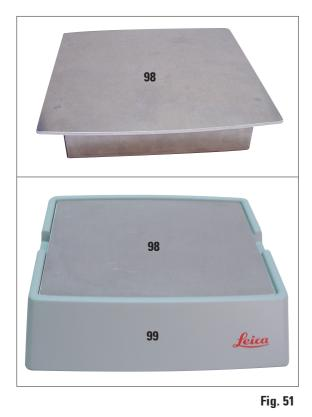
The tray is mounted on the hood of the microtome so that the small feet on the underside fit into the cutouts on the hood.
