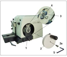
The feather key (4) is loosely placed in the handwheel shaft (1) and fixed in place with a tie-rap during transport.
