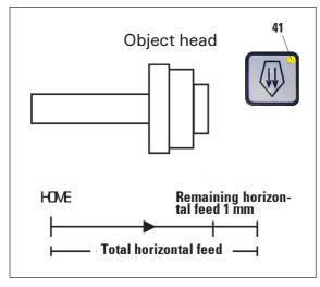
The visible and audible remaining feed indication feature informs the user during trimming and sectioning when a remaining feed of approximately 1 mm is available before the front limit is reached.
