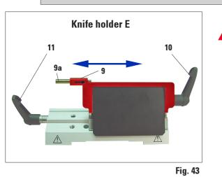
The clamping levers on the knife holder are not interchangeable. The two clamping levers (10, 11) must remain in the position shown at all times, as otherwise isolated malfunctions of the knife holder can occur. Clamping lever for the blade (10) at the right, clamping lever for the lateral displacement (11) at the left.
