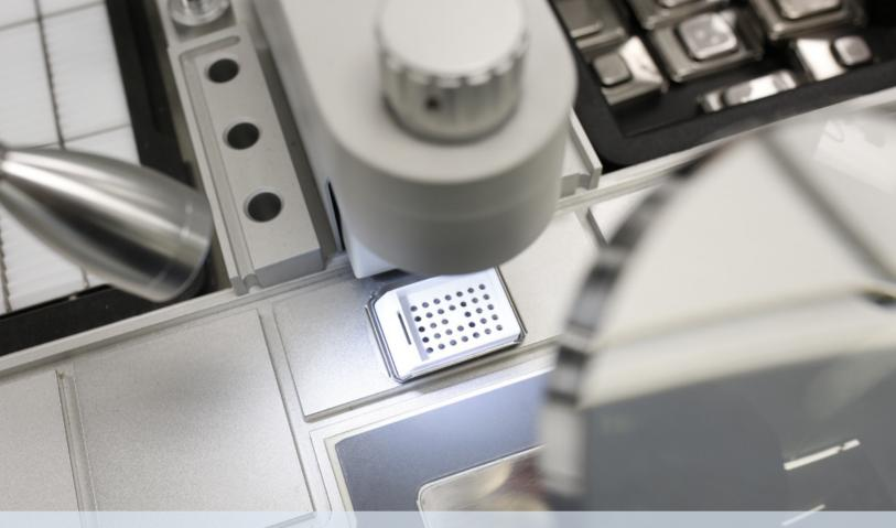
A built-in LED work light on a flexible arm comes as a standard feature, giving you total control of your lighting. The brightness can be adjusted to your preference for optimal specimen visibility.
