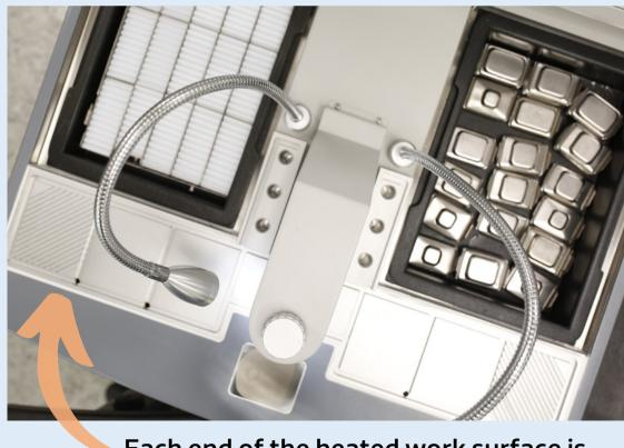
Each end of the heated work surface is ribbed for convenient block trimming
