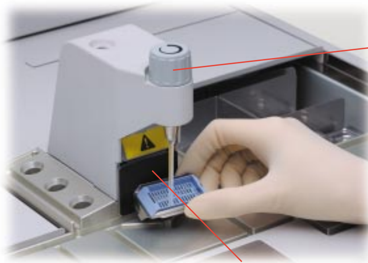
Finger touch plate and optional foot switch control the paraffin flow
