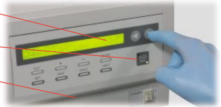
Precisely metered and adjustable gravity-feed paraffin dispenser delivers the right amount of paraffin from the 4-liter Paraffin Chamber
