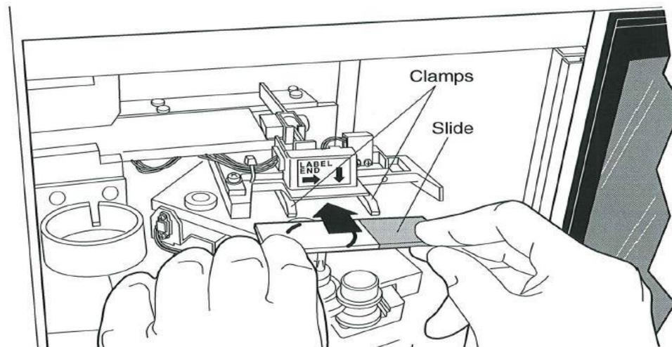
The slide should now rest *on top* of the two clamps and *under* the upper guide block.
