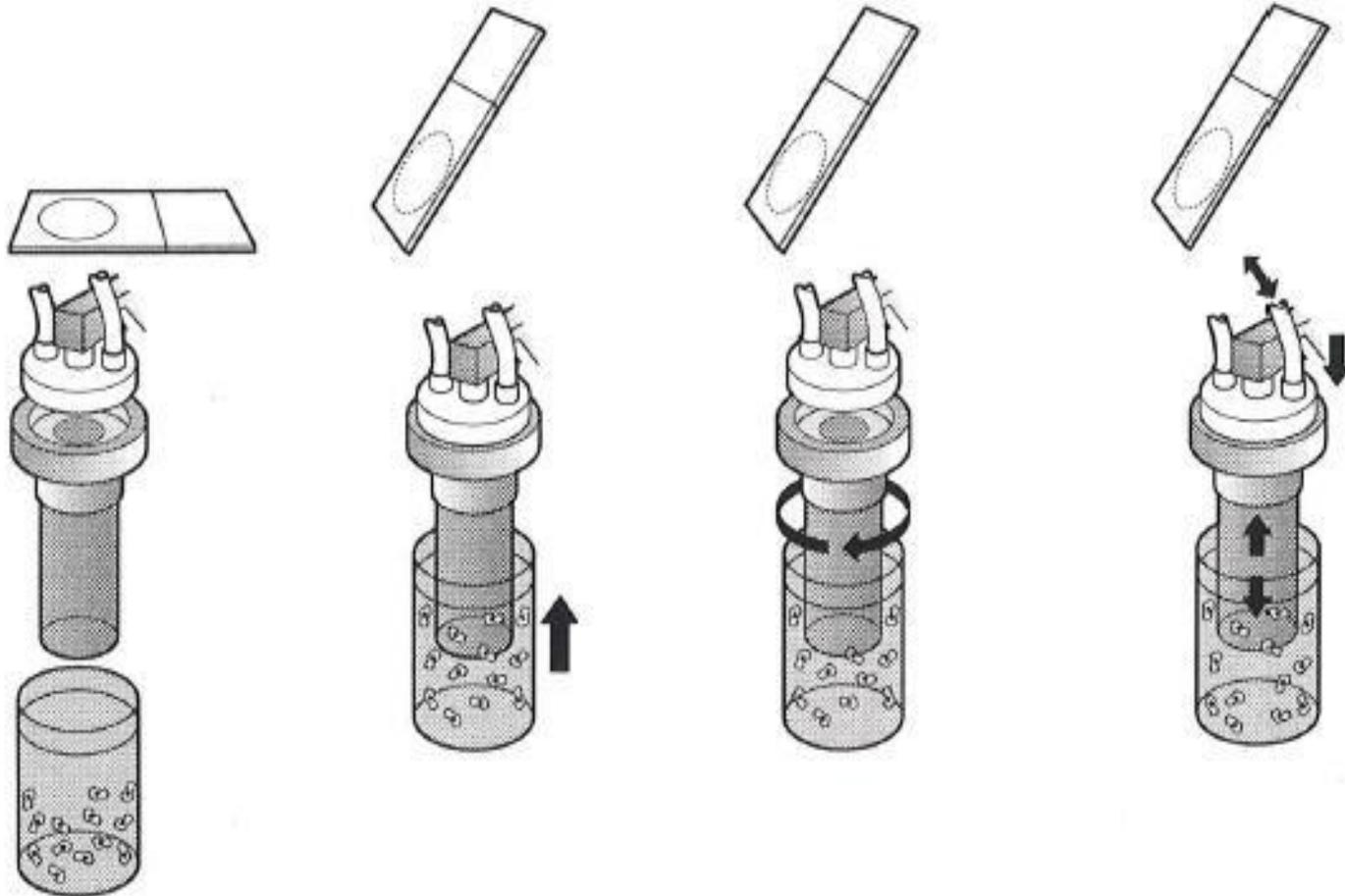
1. Slide and TransCyt Filter are in place. Operator initiates sequence.
