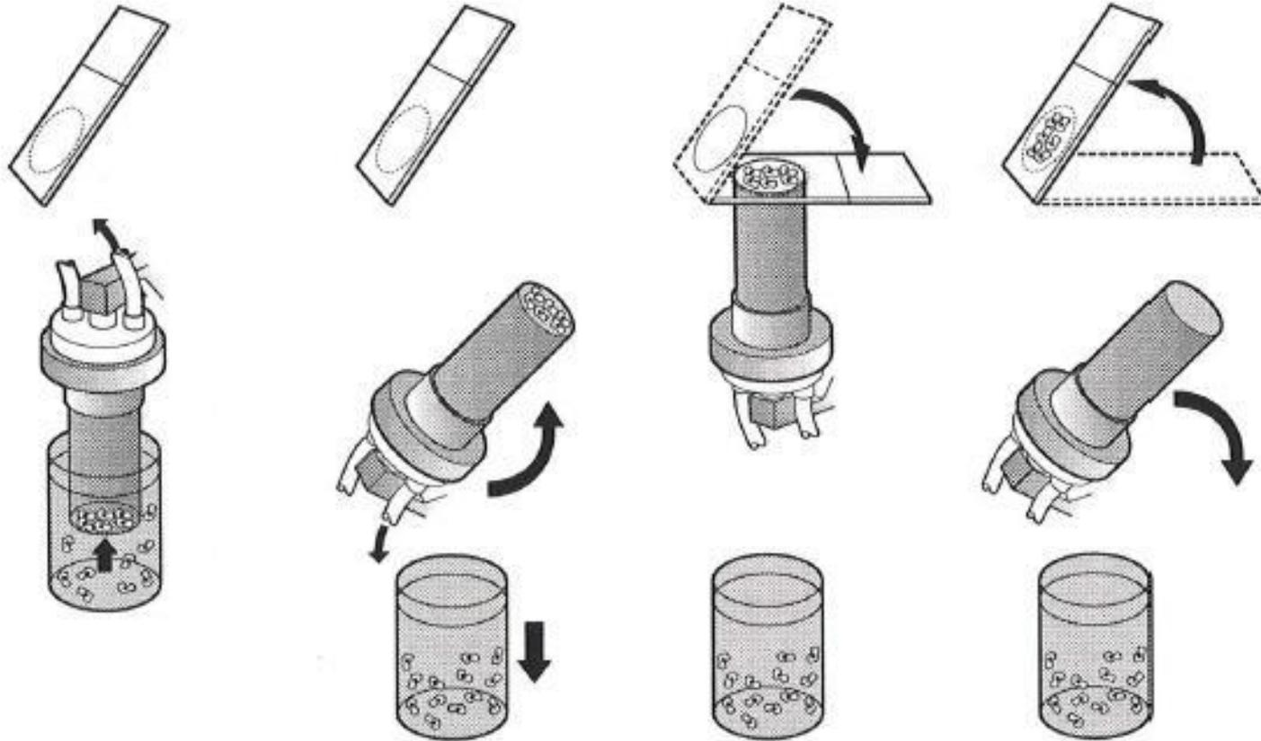
5. Collection. Sample is drawn onto TransCyt Filter in a controlled manner.
